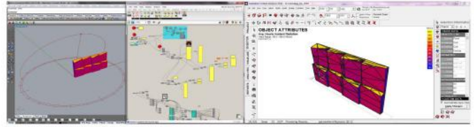
Rhino 3D and Grasshopper pluggins with Geco linking Ecotect
