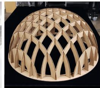
CREATE AND ASSEMBLE FORM-WORK
